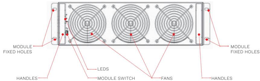
For the UPS, modules must be inserted to make a complete UPS system. The replacement of UPS module is very simple and can be operated online. The control system of the UPS can detect the inserted or removed module (s) automatically. The user may operate easily by following the steps mentioned below.
