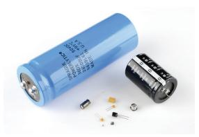
Capacitors are enclosed in aluminium or chromium- plated cylinders and contain a pair of conducting surfaces, typically electrodes or metallic plates. A third element, known as the dielectric medium, separates and insulates these elements.
