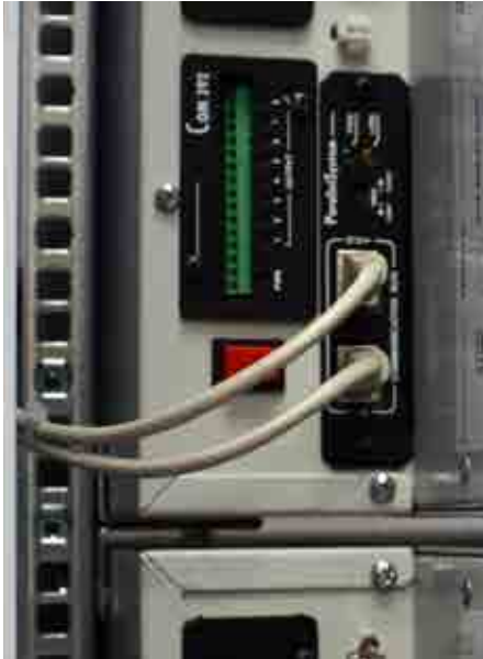
Parallel configuration and programmable relay contacts board.
