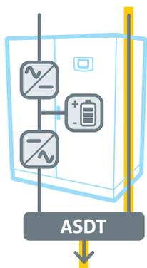
In the event of power supply failure the internal automatic device (ATSD) transfers the load to the inverter. The battery provides power to the inverter, ensuring the required runtime.
